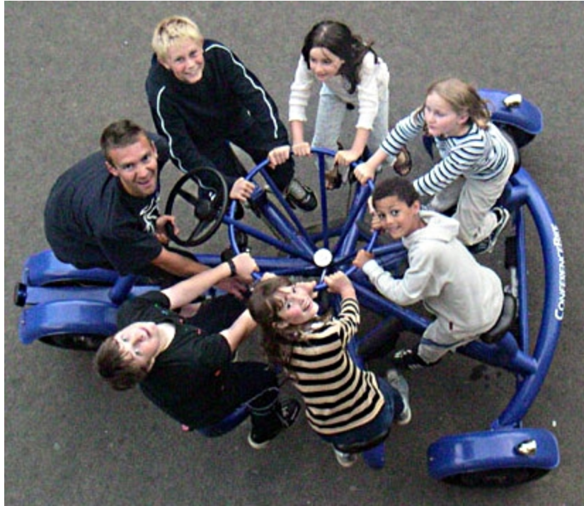
Eric Staller's ConferenceBike (CoBi) is a circular bicycle built for 7-people to peddle and one-person steer
